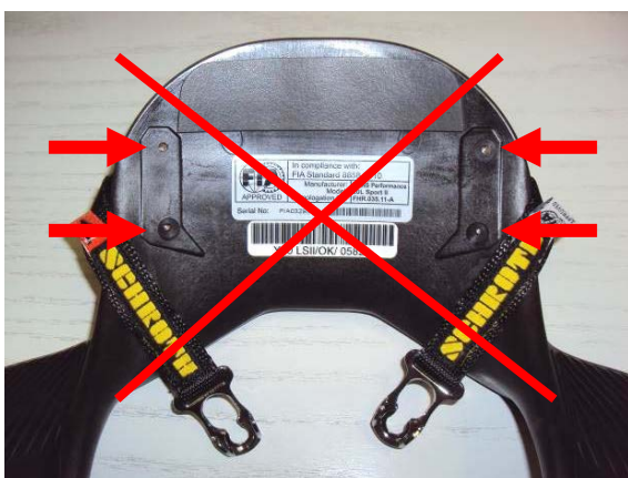
Figure 1 – Without screws fixing the tether carriers part must not be accepted
